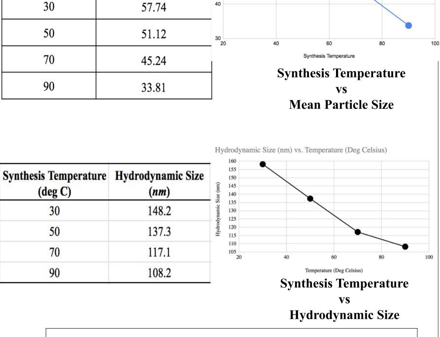
Both particle size and hydrodynamic size decrease as synthesis temperature increases consistent with the equation below
