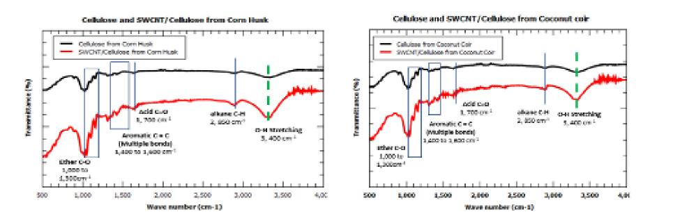
Photographs, SEM and FTIR results revealed that nanotubes can be dispersed in a solution with the use of cellulose extracted from corn husk and coconut coir.
