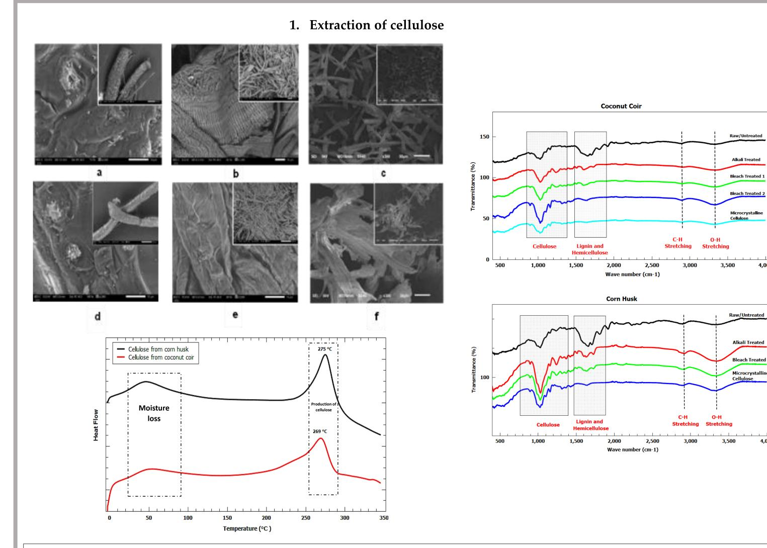
SEM, FTIR and DSC results implied the removal of hemicellulose, lignin and other impurities present in fibers both in corn husk and coconut coir, and microcrystalline cellulose was obtained
