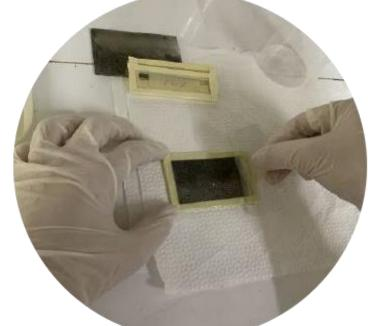
Application of PU-Urea hybrid coating on the metal substrate
