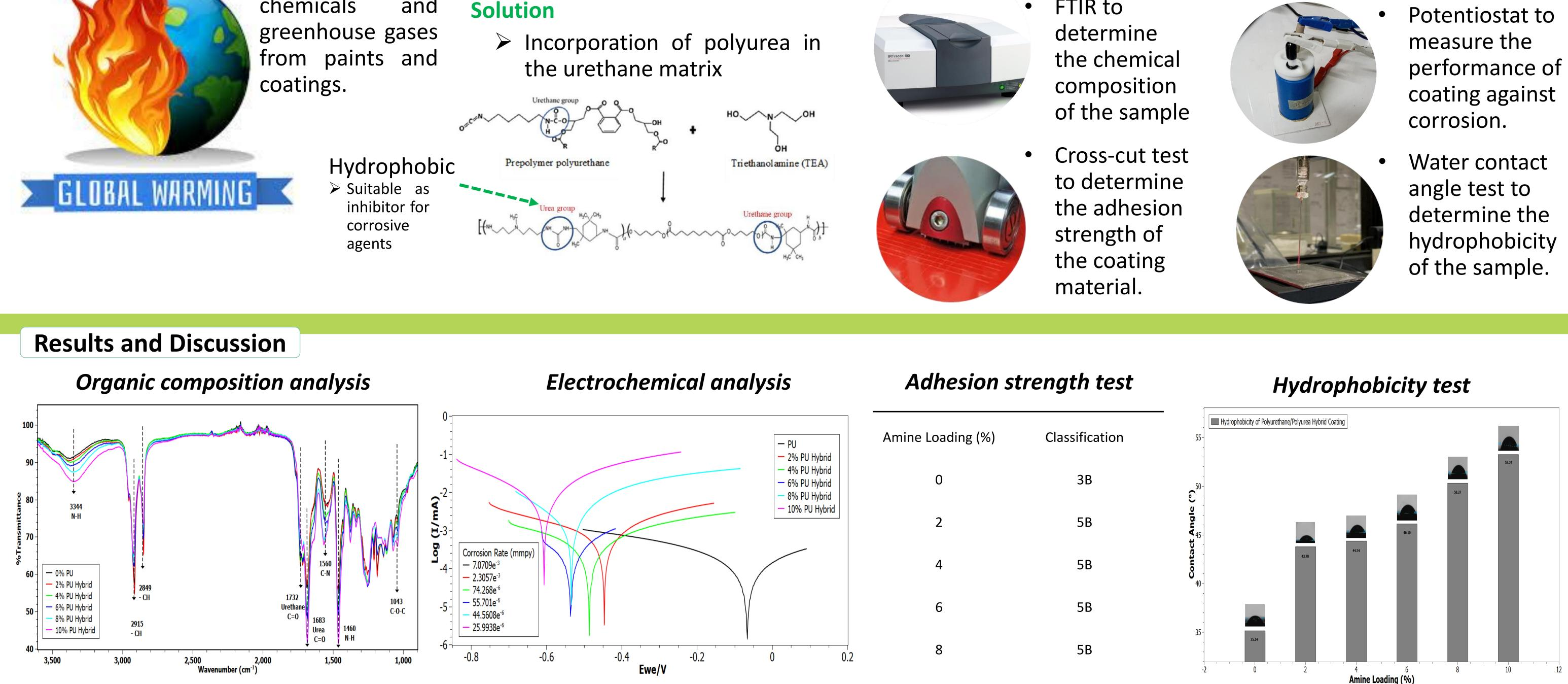
The FTIR spectrum of Poly(urea)urethane Hybrid shows signals in the peak of 3344 cm<sup>-1</sup> which are the results of symmetric and asymmetric stretching vibrations of the N-H groups present in urethane derivatives.
