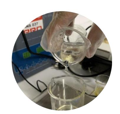
Pre-polymerization of PU and incorporation of TEA and addition of NCO to form PU.
