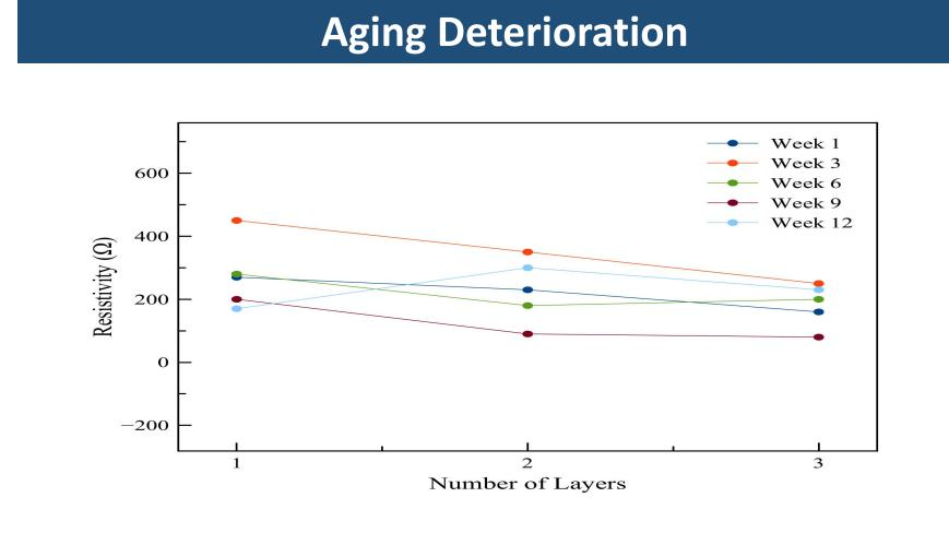
Resistivity of the pure graphite film examined every after three weeks for three months does not degrade over the span of time significantly.
