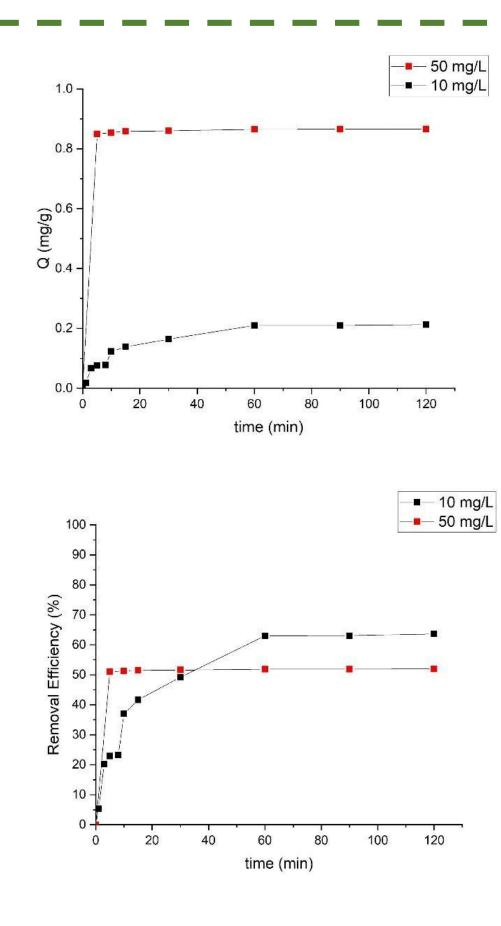
The removal efficiency and adsorption capacity (Q) of PUAC composite increased over time until they reach a maximum, as illustrated in the figures on the left. The removal percentage obtained both concentrations are similar suggesting that the PUAC can still absorb Pb at concentrations. higher Moreover, the quantity of the pollutant adsorbed per unit of mass of adsorbent increases with the increase of the concentration of the solution.
