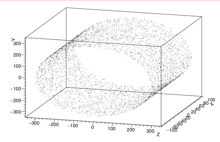
The distribution of the annihilation photons as detected by the PET detector following a 150 MeV/u carbon ion irradiation of the water phantom.
