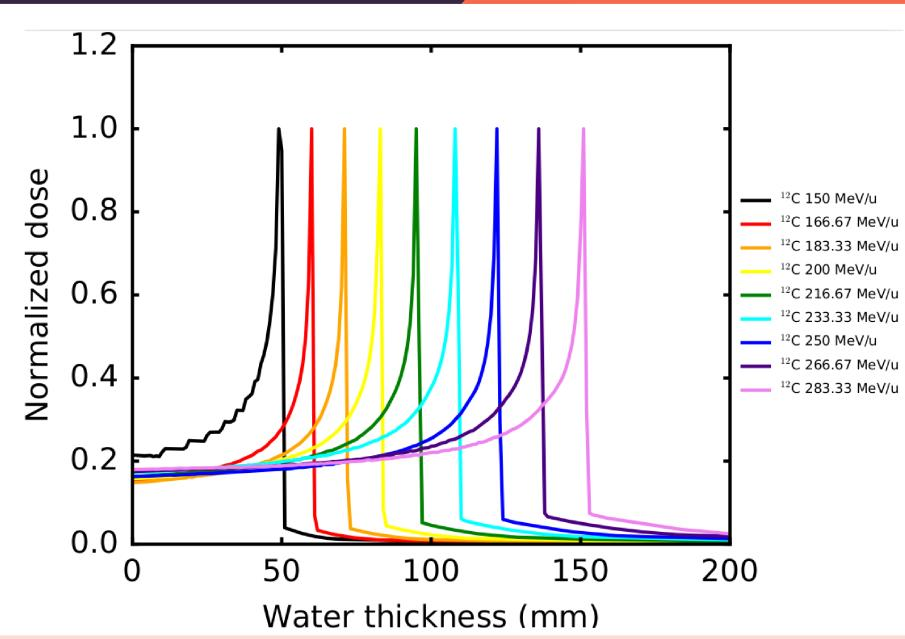
The incident energy of the carbon ion beam is varied uniformly from 150 MeV/u to 283.33 MeV/u. As the incident energy of the beam increases, the Bragg peak is found at a deeper location within the medium.
