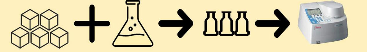
1.5 g of PUAC was added to a 50-mL stock solution (100 & 200 ppm) and shaken at 100 rpm
