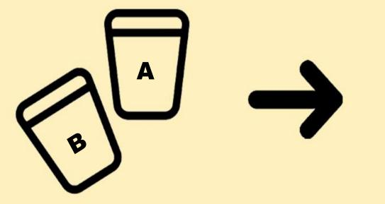
Component A (catalyst, surfactant, polyol, and filler) was mixed with component B (MDI)
